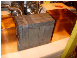
Installation of the shielding for the Sunset Micromegas
