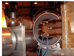
Back view of the Sunrise Micromega before closing the inner shielding
