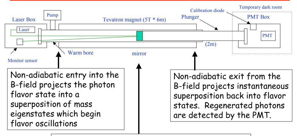
A mirror projects the transmitted wave into pure axion flavor. This transmitted superposition of mass eigenstates again begins oscillations in the region beyond the mirror.
