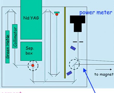
Laser box is safety interlocked, mounted on cement blocks, and interfaces to vacuum inside the magnet.
