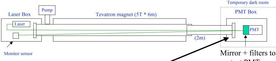
A vacuum window (outside of the magnetic field) projects the transmitted wave into pure photon flavor and the reflected wave into pure chameleon flavor.
